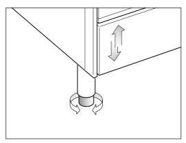
Figure 5 Levelling the cooker
